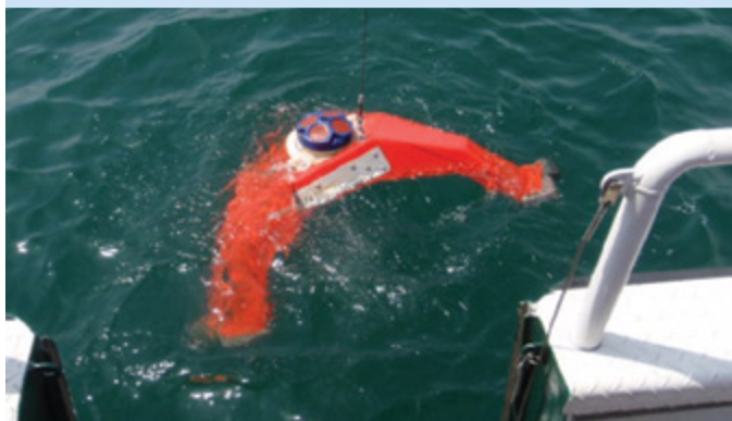
FIGURE 2.2: Deployment of an Acoustic Doppler Current Profiler (ADCP) on the lakebed of Lake Ontario for the 2009 survey season
